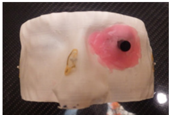
Figure 4B: The patient phantom shell after the dummy tungsten shield was placed and the simulated wax eyelid added.
