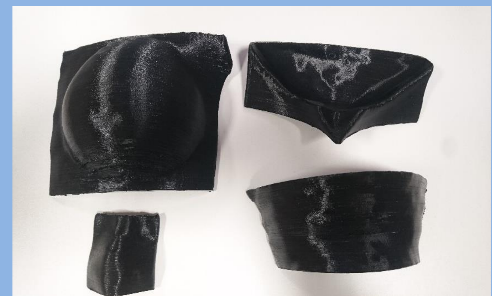
Examples of 3D printed bolus
