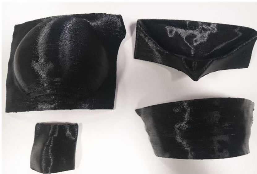
First 3D printed boluses created at SLRON: Upper left: breast; upper right: vulva; bottom left: nose; bottom right: neck.
