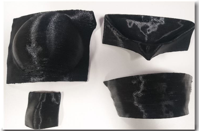
Figure 2. First 3D printed boluses created at SLRON: Upper left: breast; Upper right: vulva; Bottom left: nose; Bottom right: neck..
