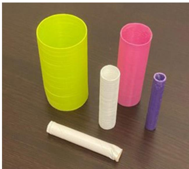
Figure 3: 3D printed cylinder spacers in comparison to cardboard tubes.
