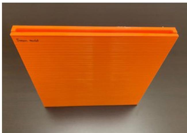
Figure 2: A 200x200x5 mm<sup>3</sup> 3D printed silicone mould for in-house standard sheet bolus production.
